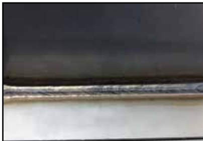
■ CrNi Kehlnaht PB | 1,0 mm POWER.ARC
