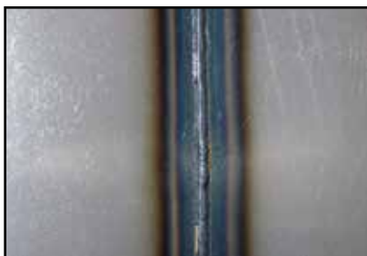
■ Stahl Stumpfnahht PG | 2,0 mm ROOT
