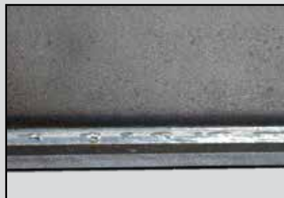
■ Stahl Kehlnaht PB | 5,0 mm POWER.PULS
