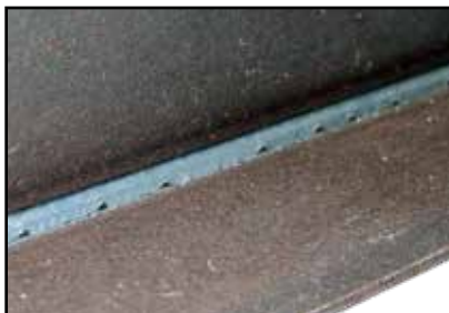
■ Stahl Kehlnaht PB | 8,0 mm FOCUS.ARC
